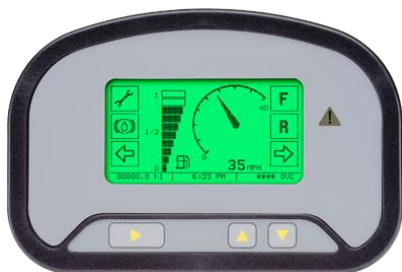
■ Curtis CAN, LED controller with EMC and water-dust prevention.
