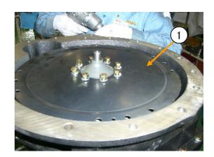
After installing, check that the height of between the flexible plate and the T/C case is about 11mm.
