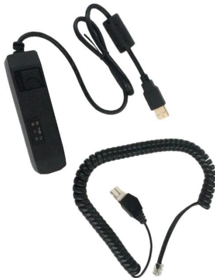
Figure 12 - Curtis Model 1314 Laptop Based Programmer
