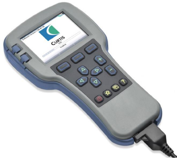
Figure 11 - Curtis Model 1313 Handheld Programmer
