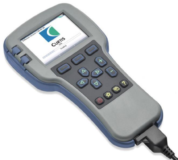
Figure 11 - Curtis Model 1313 Handheld Programmer
