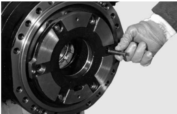
FIGURE 17: Remove the reversal springs (9) and screws (10).
