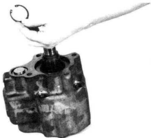
Figure 29 Remove piston bore plug retainer ring.
