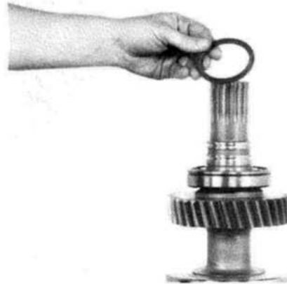
Figure 55 Remove rear bearing washer.
