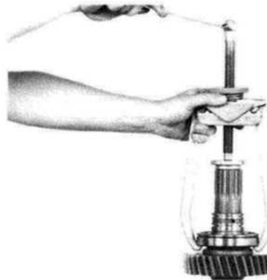
Figure 56 Remove rear bearing.
