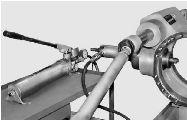
FIGURE 19: Connect the tension bar to the press and push the thrust blocks of bearings (9, 10) into their seats. Disconnect from the press and remove tension bar and drivers.
