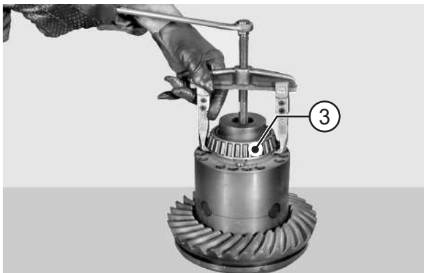
FIGURE 2: Using a puller, remove bearing (3).
