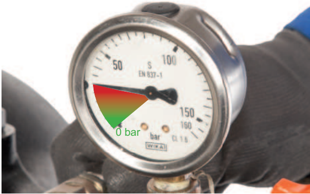
FIGURE 11: Gradually release the pressure in the braking circuit, bringing it to zero through the external pump.
