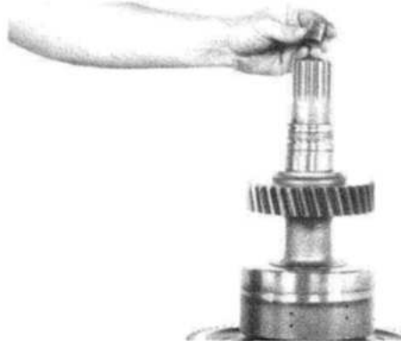
Figure 57 If P.T.O. shaft front bushing is to be replaced, remove bushing.
