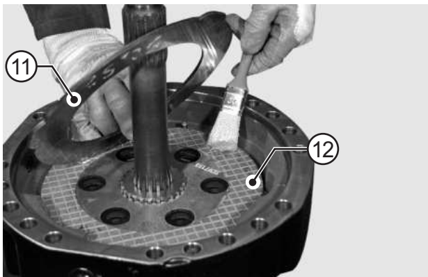
FIGURE 47: Insert the brake discs (11, 12) in the right sequence.
