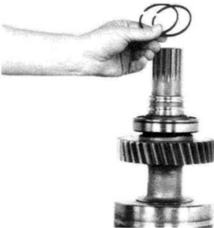
Figure 53 Remove clutch shaft oil sealing rings.
