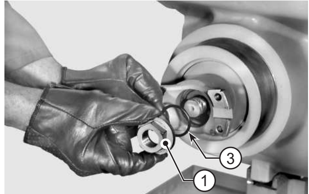
FIGURE 4: Remove nut (1) and o-ring (3).
