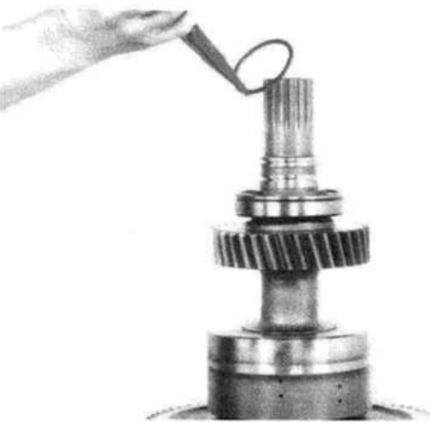
Figure 54 Remove clutch shaft rear bearing retaining ring.
