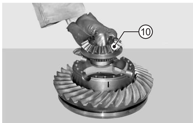
FIGURE 6: Remove the 2nd planetary gear (10).
