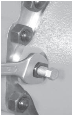
FIGURE 1: Loosen nuts (22) of screws (23) provided for the mechanical and manual release of the braking units, then move the nuts backwards.
