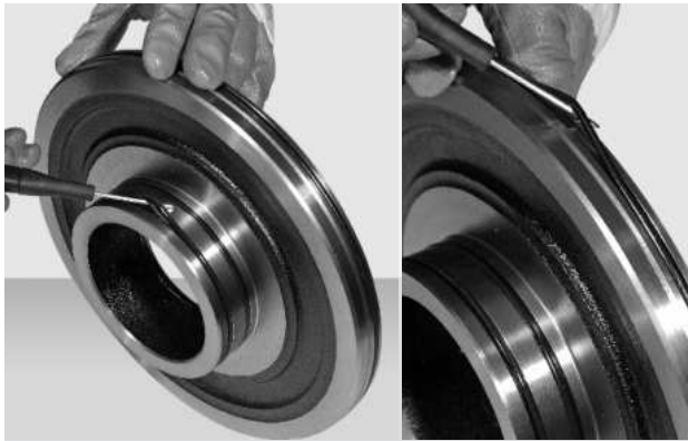
FIGURE 24: Fit antitwist rings (2, 4) onto the piston (3).
