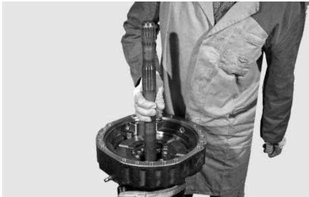
FIGURE 2: Remove the axle shaft.
