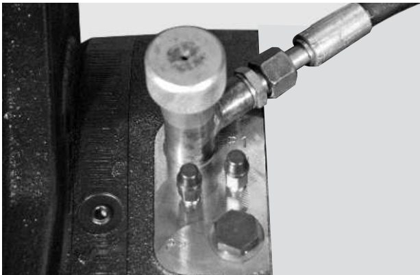
FIGURE 12: Gradually loosen the sleeve and remove.
