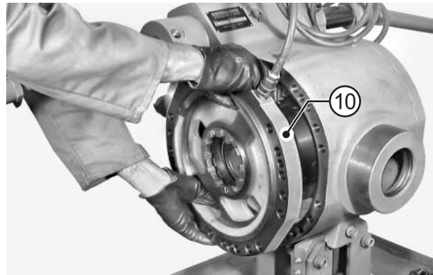
FIGURE 39: As you hold the selector fork in position (16), rotate the intermediate cover into its final position (10). To lock into position, tighten two safety studs "A" in two opposing holes.
