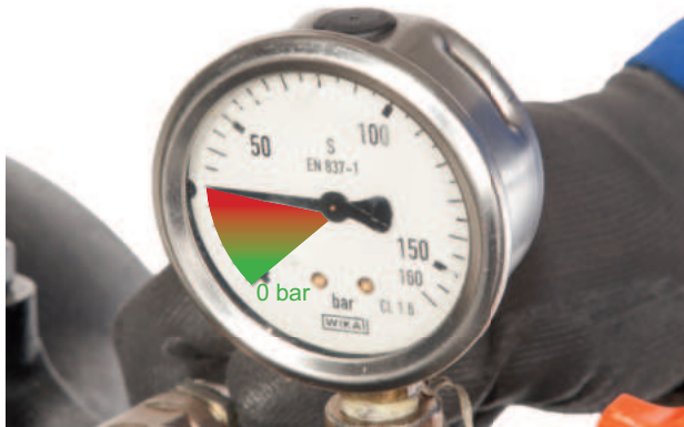
FIGURE 52: Gradually release the pressure in the braking circuit, bringing it to zero through the external pump.
