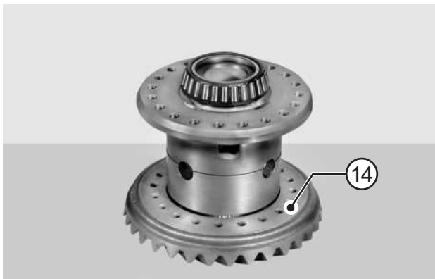
FIGURE 12: Remove the ring gear (14).
