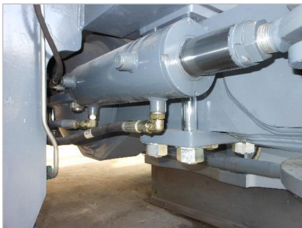
Typical position of steering cylinders front and rear axles
