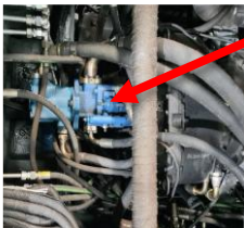
Main Hydraulic Pump: The system uses a variable displacement vane pump to supply fluid to the hydraulic system under normal operating conditions. The pump is directly coupled to the transmission's PTO drives and is fed from the oil reservoir through individual flooded suction lines to ensure consistent fluid supply. It is self-compensating, automatically adjusting its output to match system demand. Refer to the Hydraulic Drawing in this manual for system operating pressures.
