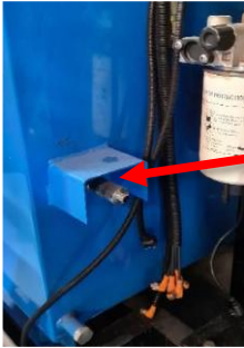
High Hydraulic Temperature Sensor: Located on the side of the hydraulic tank and provides warning if the hydraulic temperature exceeds 70 deg. C.
