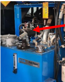
DC Pump: An electric powered hydraulic pump that is used in the event of an emergency e.g. failure of main hydraulic pumps (engine driven), Engine failure or any other scenario that may occur that requires hydraulic power.
